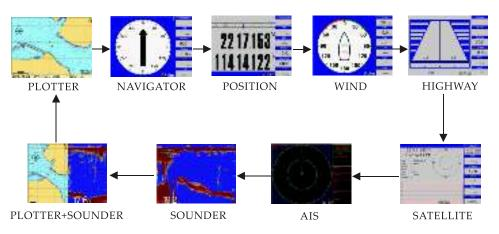
Press the [MODE] key to choose a display mode. Each time the key is pressed, the display mode changes in the sequence shown above.
